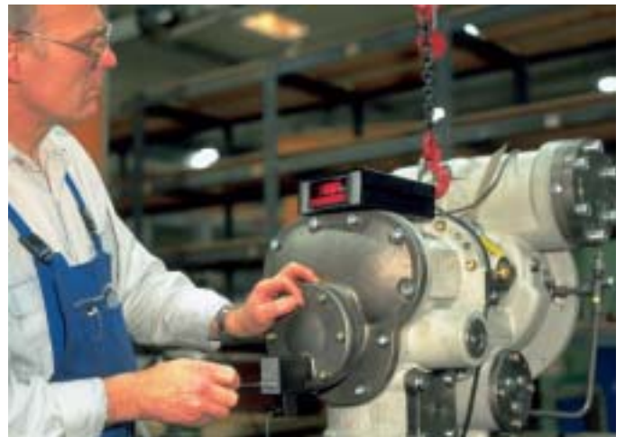
Preparing for the test run of a screw compressor. All compressors are test run and all packaged units are pressure and leak tested prior to delivery according to the selected manufacturing standards.
