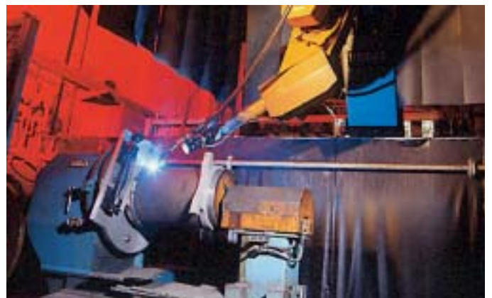
Welding robot. Manufacturing of Grasso's unique welded steel reciprocating compressor crankcase
